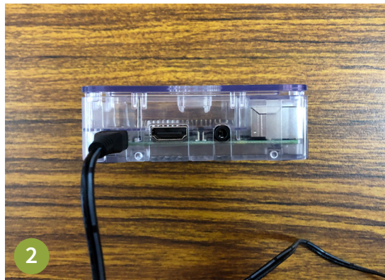
1. & 2. Step 1: Attach the included power supply cord onto the Raspberry Pi and PLUG the other end into a power source. 3. Step 2: A flickering green light and constant red light should appear on the device indicating that it’s powering on and booting up. Now you’re ready to log on to Wi-Fi settings, look for ‘Moodlebox’ to PLAY. It’s that simple! Photo Credit: Dr. James McConnell.
