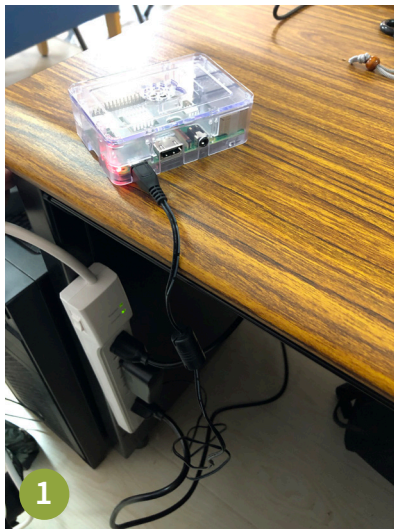
1. & 2. Step 1: Attach the included power supply cord onto the Raspberry Pi and PLUG the other end into a power source. 3. Step 2: A flickering green light and constant red light should appear on the device indicating that it’s powering on and booting up. Now you’re ready to log on to Wi-Fi settings, look for ‘Moodlebox’ to PLAY. It’s that simple! Photo Credit: Dr. James McConnell.
