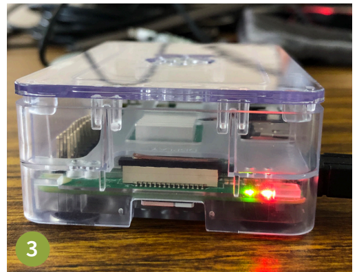
1. & 2. Step 1: Attach the included power supply cord onto the Raspberry Pi and PLUG the other end into a power source. 3. Step 2: A flickering green light and constant red light should appear on the device indicating that it’s powering on and booting up. Now you’re ready to log on to Wi-Fi settings, look for ‘Moodlebox’ to PLAY. It’s that simple! Photo Credit: Dr. James McConnell.
